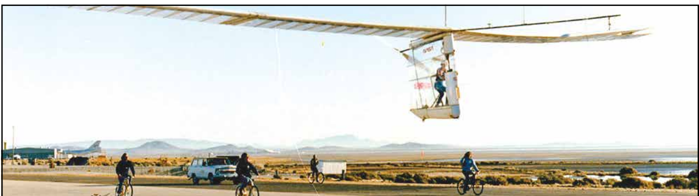
The Gossamer Condor was the first human-powered plane. (Photo courtesy of Minter Field Air Museum)
